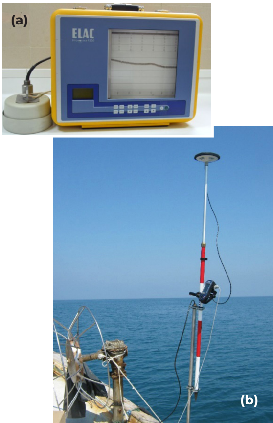
Figure 2. (a) ELAC Hydrostar 4300 Single Beam Echo Sounder (b) Bathymetrical survey of the seafloor. (Source: MCR-IOE-UOB)
